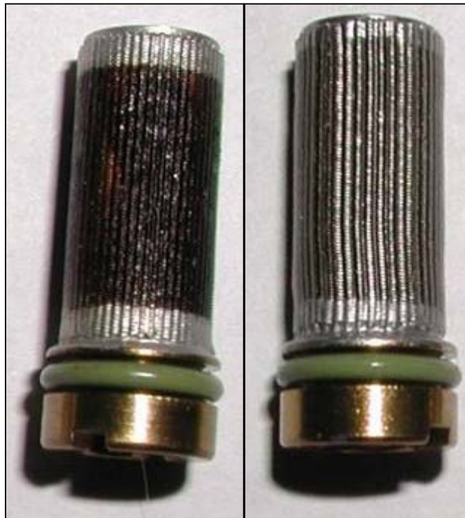
Fig 5,6. Last-chance filter from a servo valve one month after electrostatic separation technology was installed in lube-oil system (right) shows only a shadow of the brown, sticky deposit that existed prior to the modification (left)
