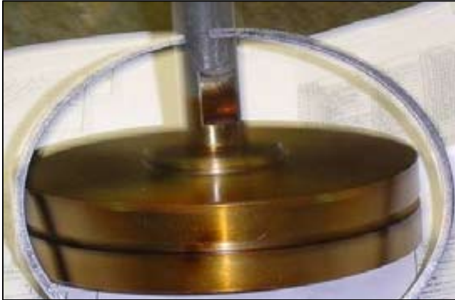
Fig 2. Varnish coating on servo-valve piston can cause part to stick or seize in normal operation
