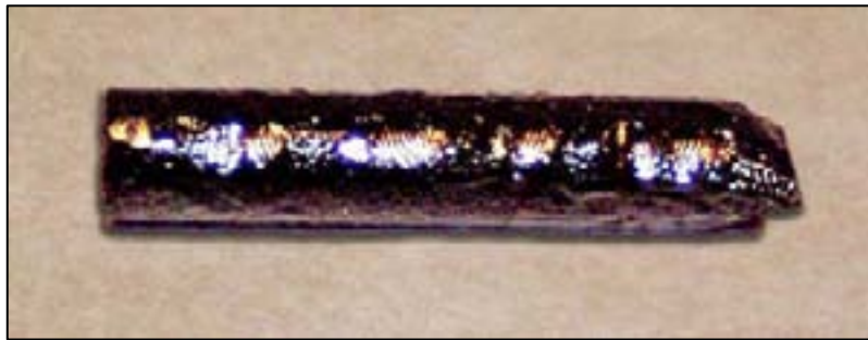
Figure 2: Heavily Varnished Pencil Strainer Inside a Fuel Oil Bypass Control Valve
