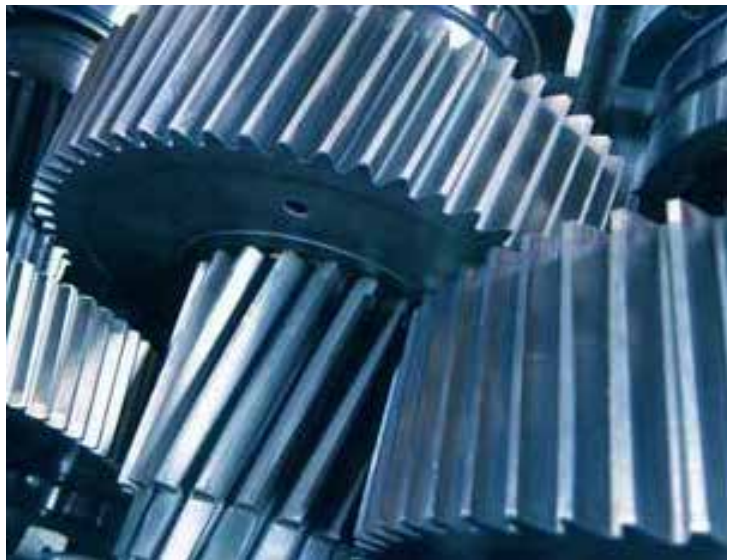
Figure 2 - Gear teeth in a wind turbine gearbox
